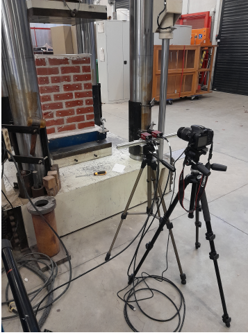
Figure 6. Experimental setup of the compression test
