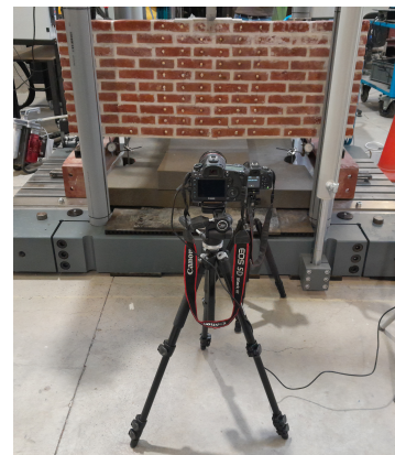
Figure 9. Experimental setup of the three-point bending test
