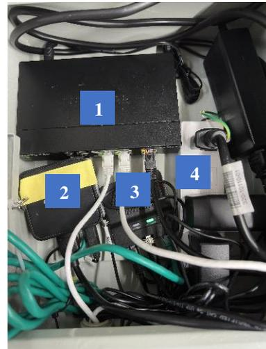
Figure 1. IP66 housing with components: 1) PoE switching hub 2) Mini computer 3) WiFi router 4) Power strip
