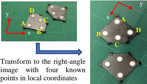
Figure 3. Transformation of targets for measuring the deformation
