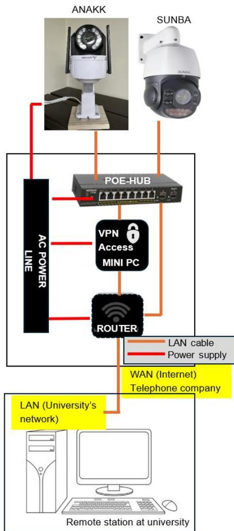
Figure 2. Remote crack monitoring system set up
