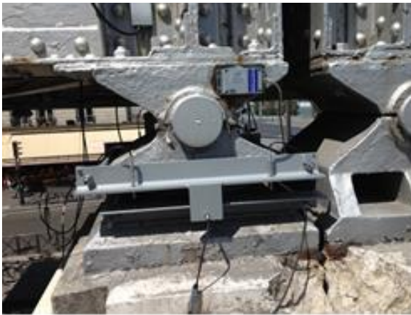
Figure 1. Picture of the bearing device equipped with relative displacement sensors
