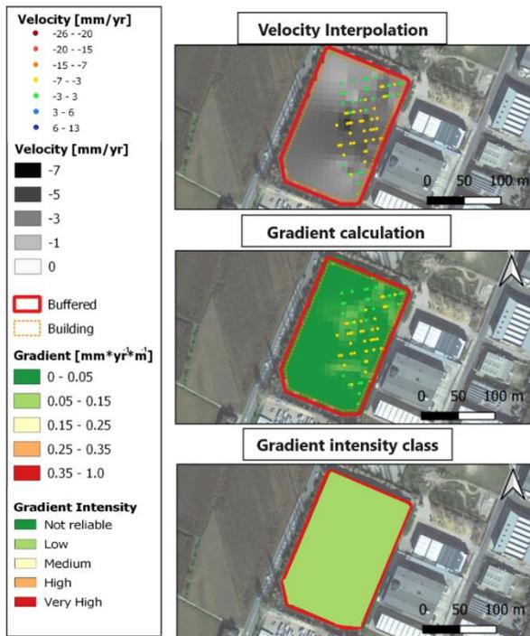
Figure 2: Deformation gradient classification starting from the EGMS MPs.
