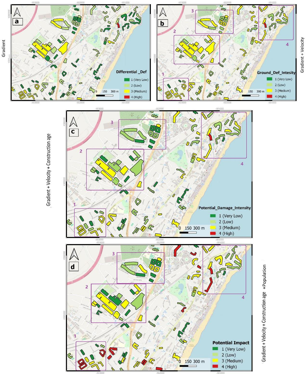
Figure 5 Case study of Torremolino. Original Differential Deformation map generated with the standard procedure (a). Three advanced products to improve the analysis: Ground Deformation Intensity map (b); Potential Damage Intensity map (c); and Potential Impact map (d).
