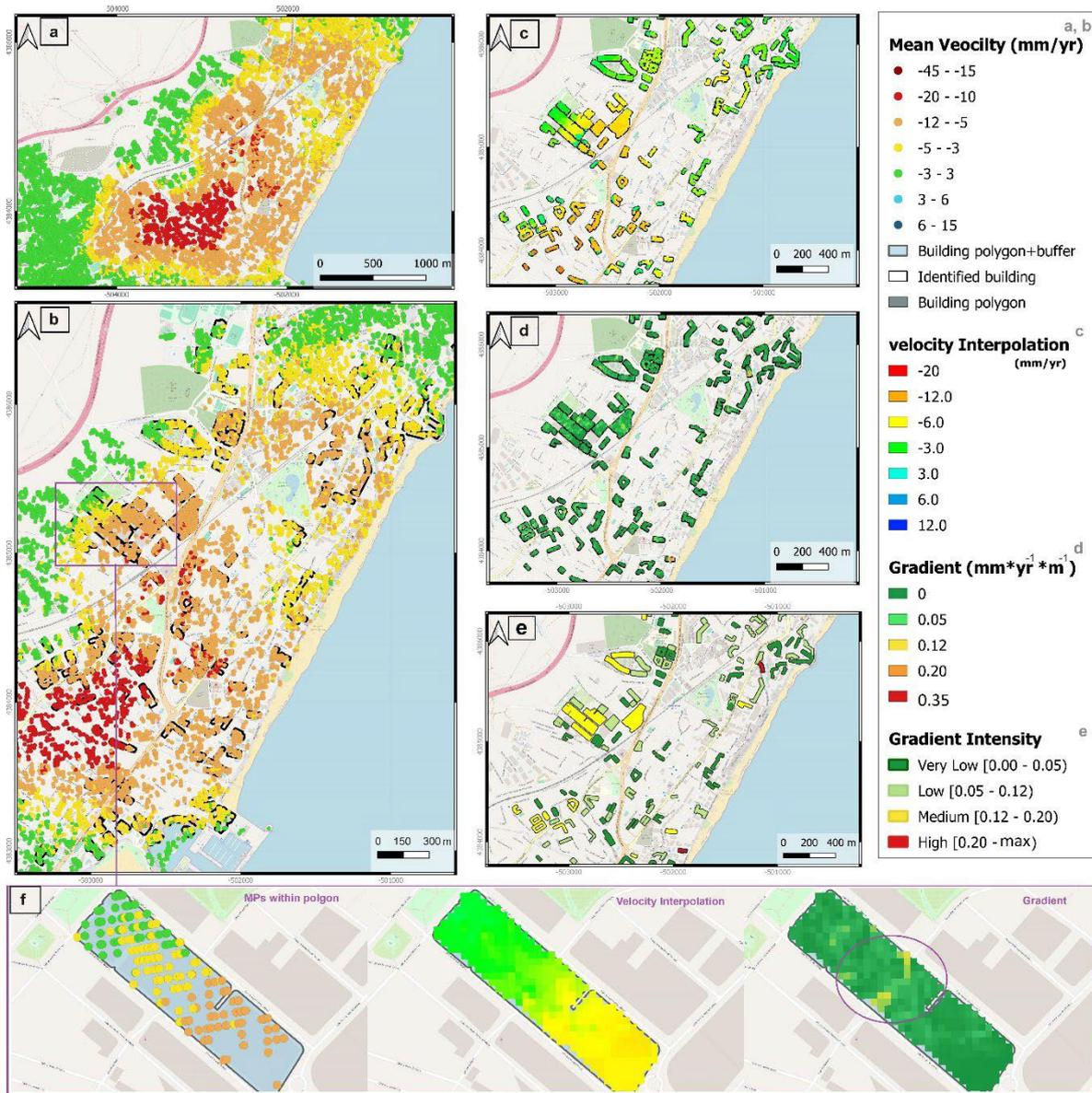
Figure 3: PSI displacement map of the town of Torremolinos (a). MPs associated with buildings (b). Velocity interpolated for each building (c). Spatial deformation gradient (d). Classification of buildings based on the deformation gradient of each building(e).
