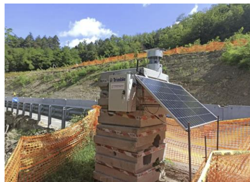
Figure 11. Dovadola site, Trimble S9 total station (Italy)
