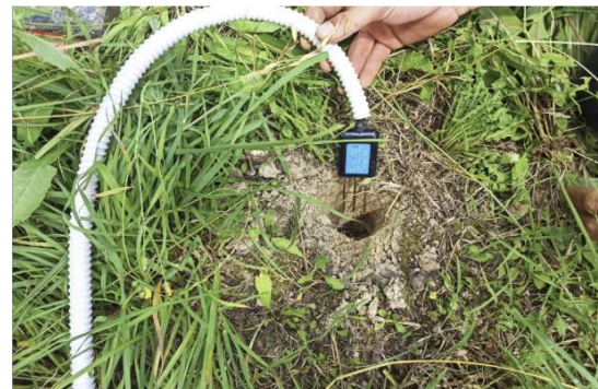
Figure 9. Monitoring system, geotechnical sensors, at Dovadola site (Italy)
