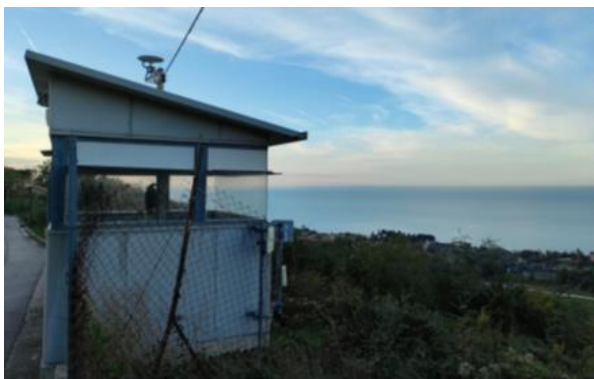
Figure 15. Monitoring system, integrated Trimble S9 total station & Trimble R750 GNSS receiver at Ancona (Italy)
