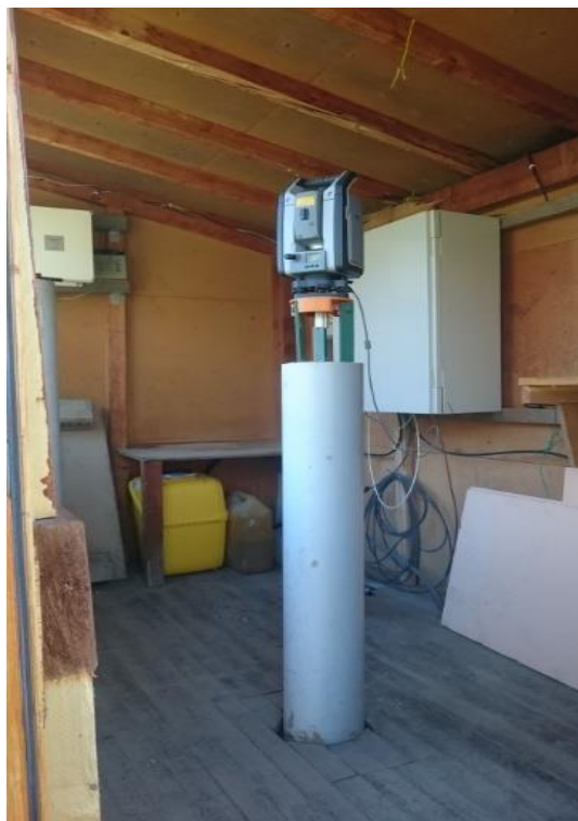
Figure 4. The Trimble S9 automated total station installed at la Valette landslide (Southern Alps, France)
