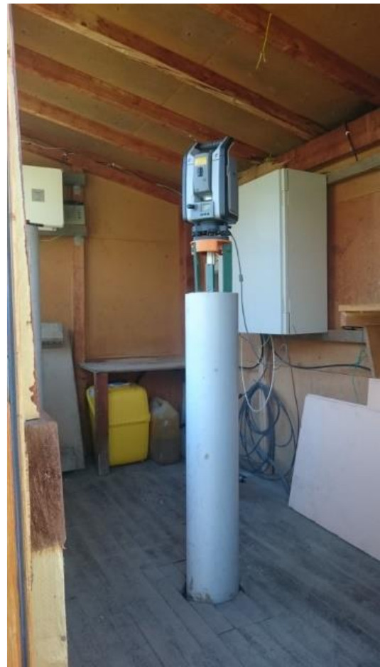
Figure 4. Permanent automated total station Trimble S9 Long Range on the pillar at the monitoring site at La Valette landslide (France)
