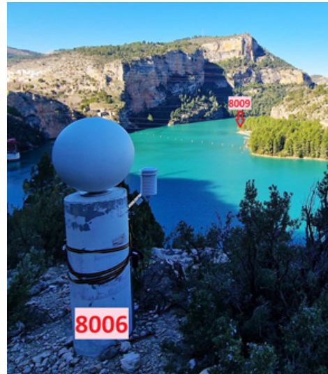
Figure 3. Pillar 8006 equipped with a \varnothing 0.5 m target sphere and a meteorological data logger used to eliminate the refraction error. Pillar 8009, which was used as TLS station in 2023 and TS station in 2024, is marked in red. The sunshade was removed for taking the pictures.
