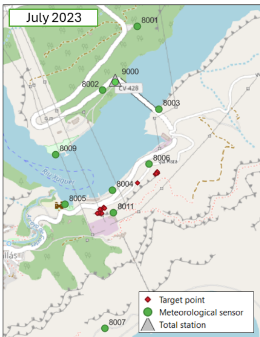
Figure 4. Locations of the involved points for the first campaign (July 2023). During this campaign, 10 meteo data-loggers were used, and both TS and TLS measurements were collected.
