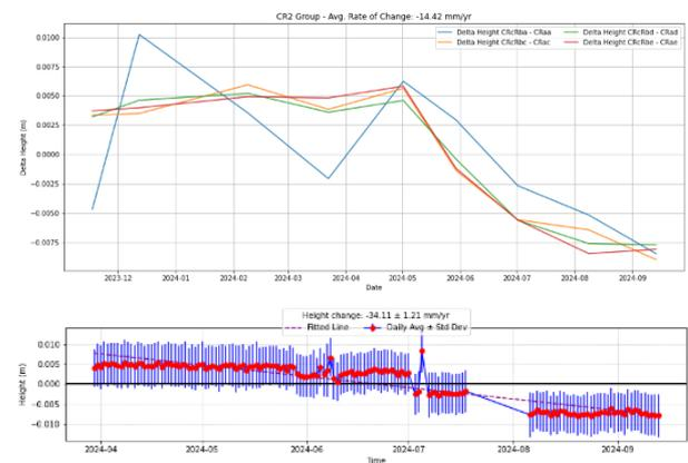
Figure 3 - GVL GNSS Height Timeseries CR2 Spen Farm Tadcaster, Top is measurements to the reflectors on the CR using a Total Station and Bottom the GVL RTK solution.
