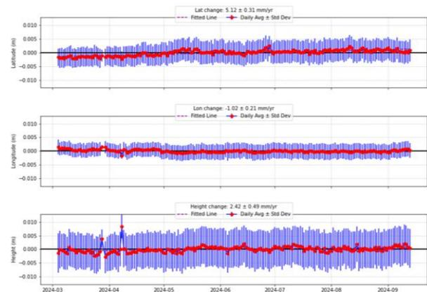
Figure 6 – GVL GNSS Time Series at Dudley Slab20
