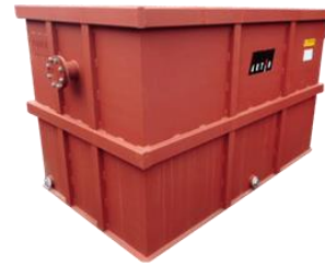
Figure 5. Test tank used for accuracy verification
