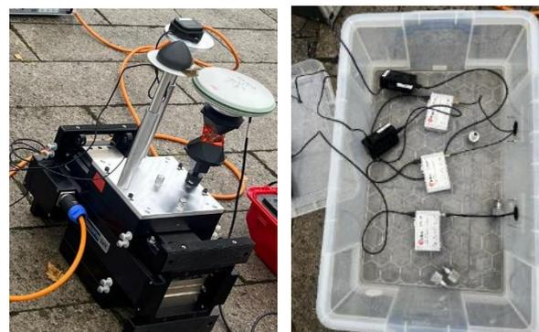
Figure 5: Left- The APS 113 shaker used for the experiment with Tallysman, Patch and Geodetic antennas. Right- U-blox F9P receivers connected to the antennas and Raspberry Pi devices to log the data.
