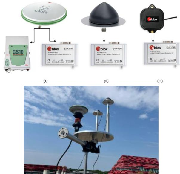
Figure 3: Top- **Experimental setup** (i) Leica AS10 geodetic antenna connected to a Leica GS10 receiver and U-Blox F9P receiver, (ii) Tallysman TWI antenna and (iii) u-blox patch antenna connected to u-blox F9P receiver. Bottom-Movement simulation device incorporated for the test.
