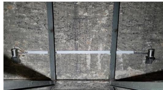
Fig. 7 View of the hydrostatic tiltmeter installed in the attics
