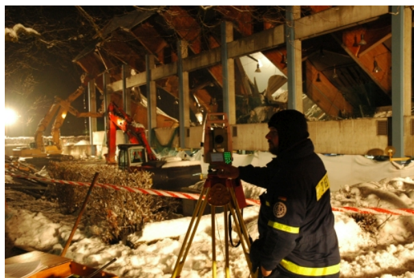
Figure 1. Monitoring at the collapsed icehockey stadium Bad Reichenhall, 4th January 2006, picture: Markus Oreck THW OV Berchtesgadener Land
