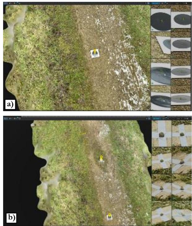
Figure 4. Determination of the (a) GCP coordinates and (b) CP coordinates, collected by iPhone LiDAR in PIX4Dmatic software
