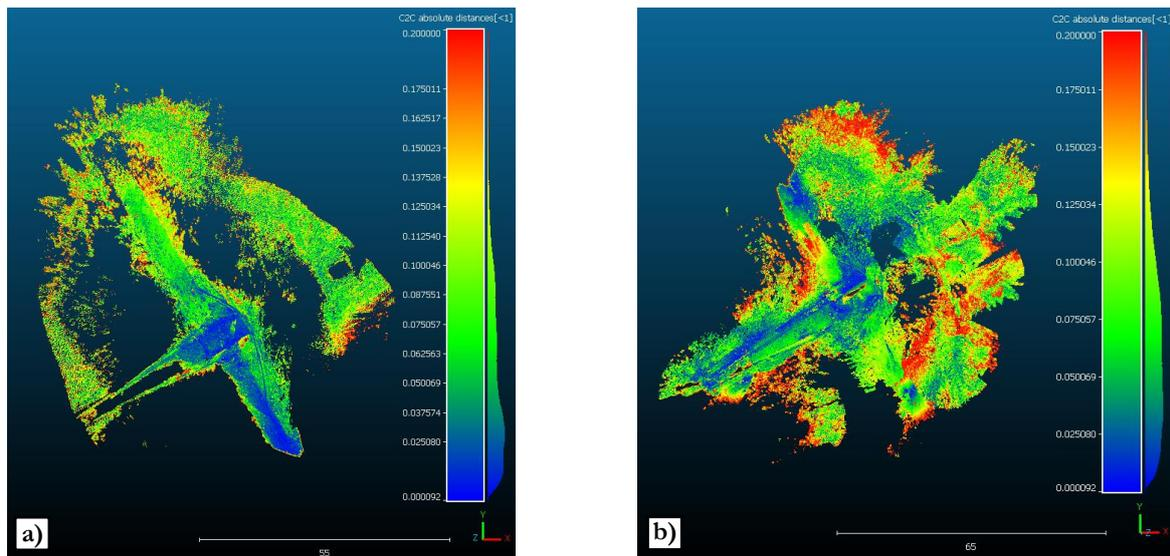
Figure 5. The display of compared point clouds obtained by iPhone LiDAR measurements on (a) the dam crown and (b) on the entire measurement area
