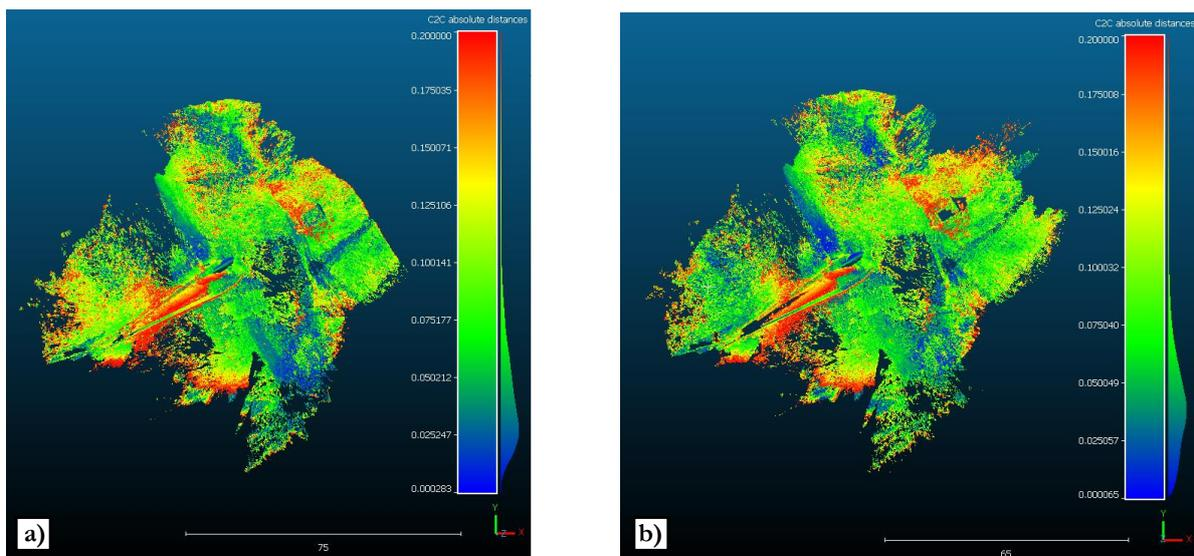
Figure 6. The display of compared point clouds obtained by iPhone LiDAR measurements with (a) UAV and (b) TLS on the entire measurement area
