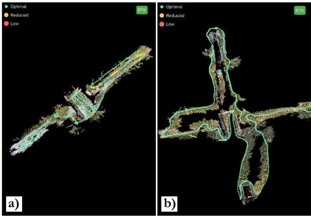
Figure 3. The display of iPhone trajectory when the survey was done: (a) from the dam crown and (b) on the entire measurement area
