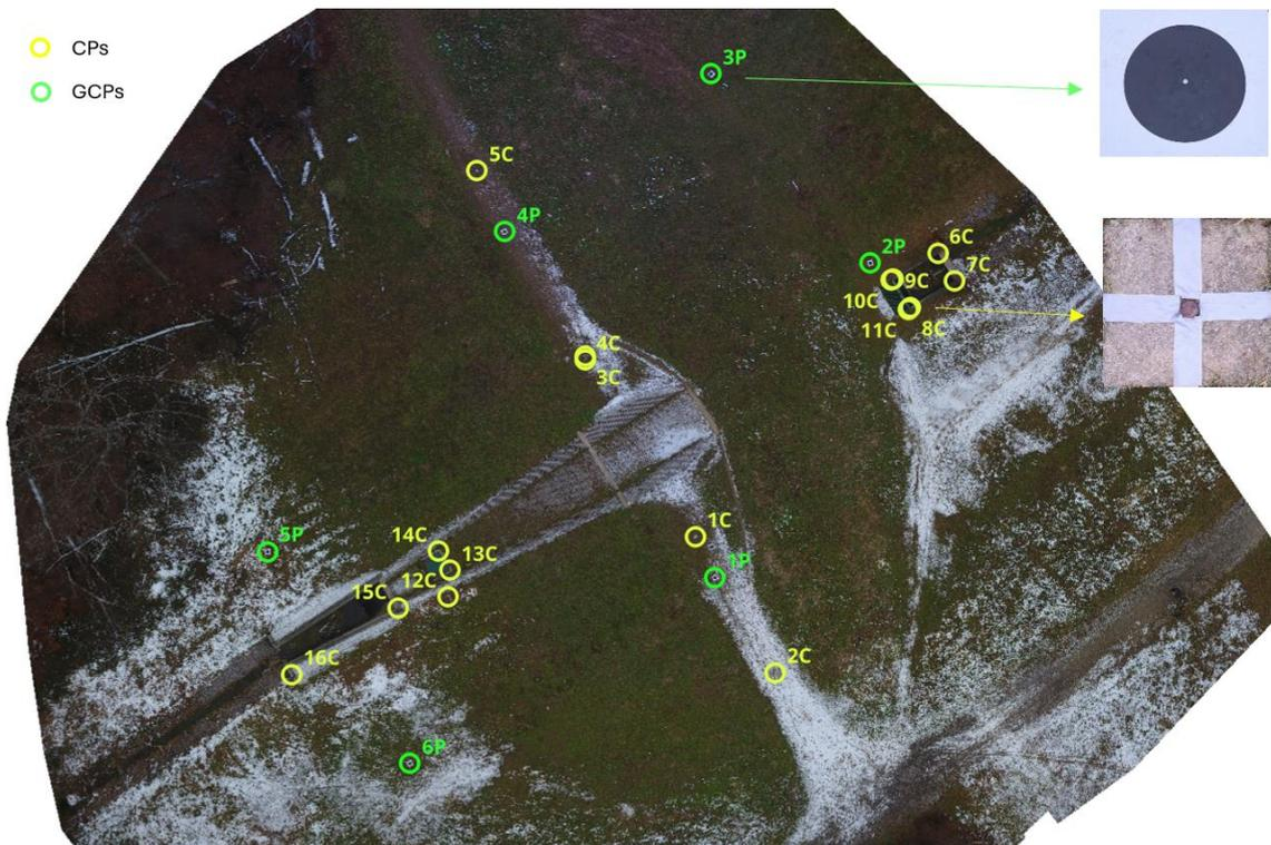
Figure 2. Orthomosaic of the embankment dam with position of GCPs and CPs and an example of point signalization for GCP 3P and CP 8C
