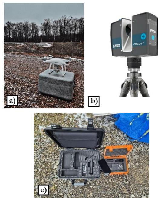
Figure 1. The measurement equipment: (a) DJI Phantom 4, (b) Faro 3D Laser Scanner S150 Premium and (c) iPhone Pro with Emlid Scanning kit (Emlid Reach RX) and viDoc RTK rover
