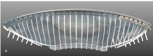
Figure 13. UAV survey of the Ridracoli dam structure lines (Buffi et al. 2017)
