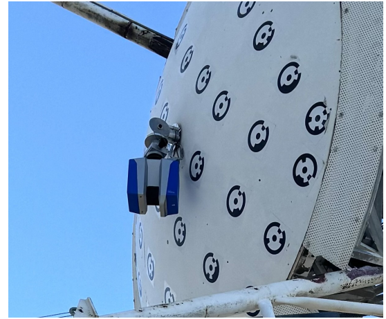
Figure 2. Scanner installation at the sub-reflector with nadir view in the scanner mounting position (HA: -89^\circ , DEC: -1.5^\circ )
