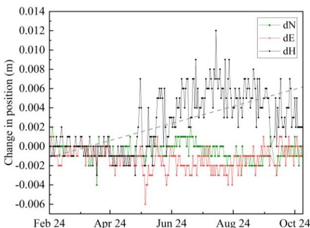
Figure 6. Change in the position for the GNSS monitoring point in Northing (dN), Easting (dE) and Elevation (dH). The dashed grey line represents the linear trend of the dH values with a slope of 10 mm/year.
