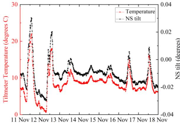
Figure 4. Variation of tiltmeter temperature and NS tilt over the span of one randomly selected week as recorded by Tilt 5. The tilt values appear to be in perfect sync with temperature.
