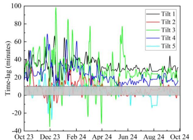
Figure 5. Time-lag between temperature and tilt over time. The grey highlighted area represents a zone where the time-lag values can be essentially regarded zero.
