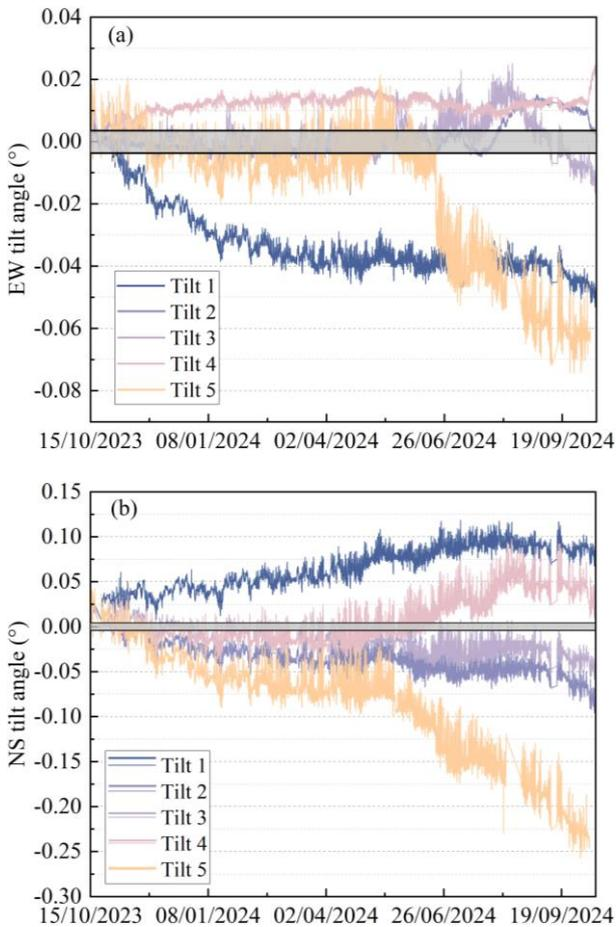
Figure 3. Calculated tilt in the (a) EW and (b) NS direction for all 5 tiltmeters. The highlighted grey areas indicate the accuracy threshold of the tilt values as calculated by eq. (1).
