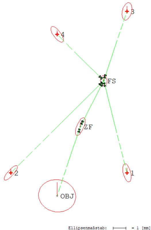
Figure 3. Result from the network simulation of free stationing with positioning of the TLS and derived object point (point cloud) with error ellipses at mm level.
