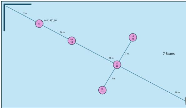
Figure 5. Experimental setup for the investigation of the distance dependence between TLS (pink circles) and total station (orange square), as well as orientation of the EOD in relation to the axis ROI (blue angle segment) - total station
