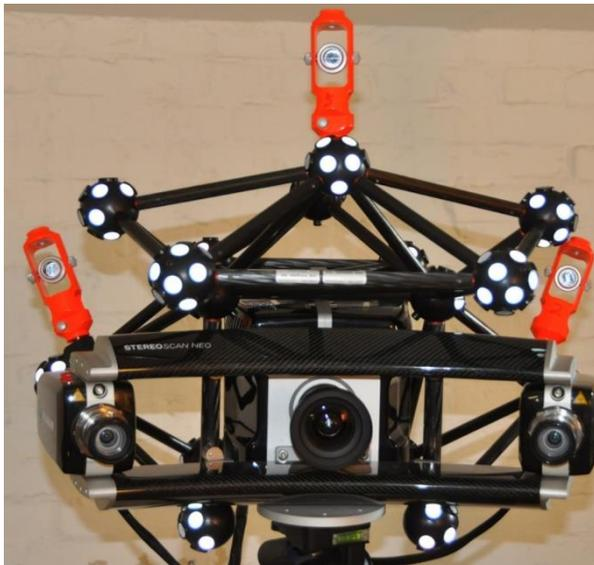
Figure 2. SLS with positioning frame and three mounted prisms
