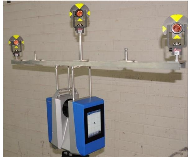
Figure 1. TLS with mounted EOD, equipped with three mini prisms
