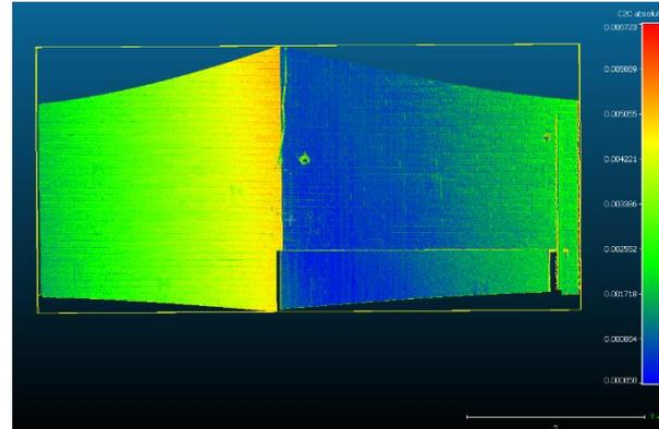
Figure 6. Comparison of the identical point cloud from georeferencing with EOD and with georeferencing using black-and-white targets. The colour scale shows the deviation of the two point clouds with a maximum of 6.7 mm in red and a minimum of better than 1 mm in blue.
