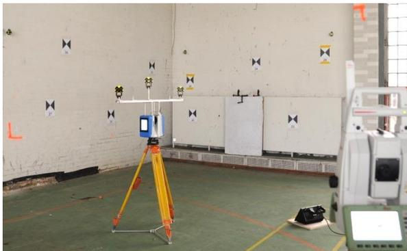
Figure 4. Test measurements with total station, TLS and the reference point field with black and white targets in the background
