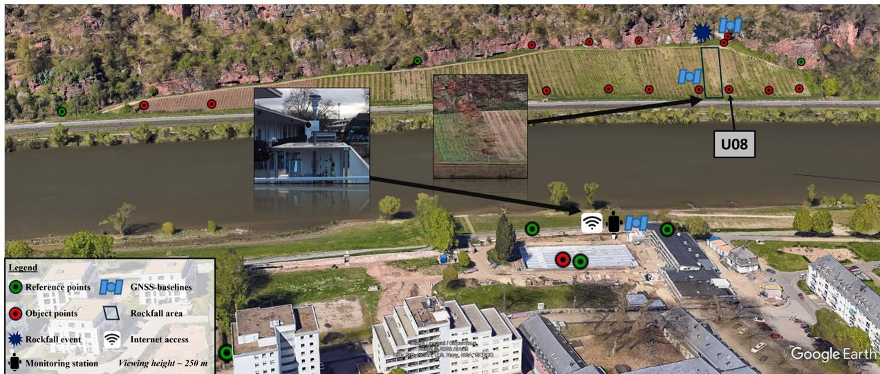
Figure 2. 3D visualization of the AImon5.0 monitoring project at the *Trierer Augenscheiner*. A potential rockfall event is automatically monitored over several years using a total station. Background map: (Google Earth, 2025)
