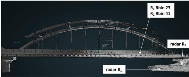
Figure 9. Three-dimensional model of the bridge with color-highlighted Rbins for radars R1 and R2, which were evaluated, and with marked positions of both radars below the structure.
