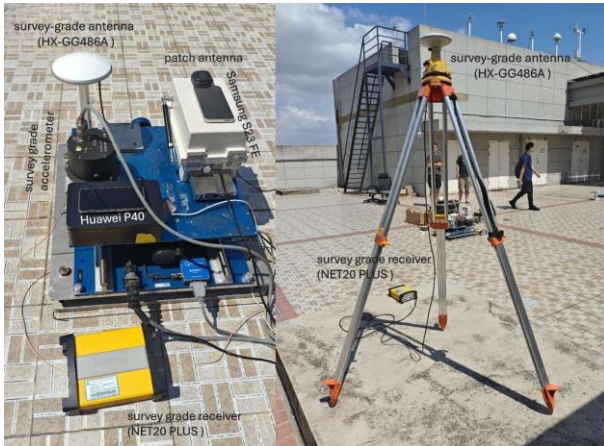
Figure 5. (left) The setup of the rover sensors (GNSS and accelerometer) on the shake table, and (right) the station consisted of survey-grade antenna and receiver
