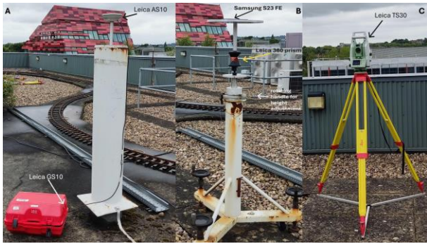
Figure 1. (left) The GNSS base station, (middle) the rover station with the prism and a metallic plate where the Samsung S23 FE has been mounted, and (right) the RTS recording the position of the prism.
